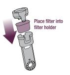
To install the assembled filter holder into the water tank, align the base of the filter holder with the adapter inside the water tank. Push down to lock into place.
